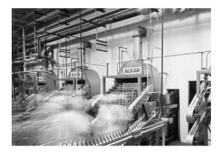
*Figure 15.16* ALKAR inline continuous cook/chill system with flow-through processing for frank-furters or wieners. (Courtesy of ALKAR, A Division of DEC International, Inc., Lodi, WI).
