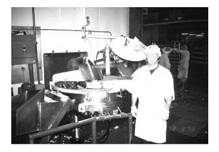
*Figure 12.2* Bowl chopper with rotating blades contained under the hooded cover at the rear of the bowl.
