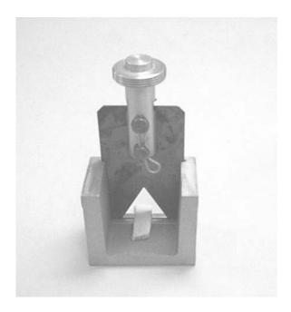
Figure 7.5 Warner-Bratzler shear cell for an Instron UTM.
