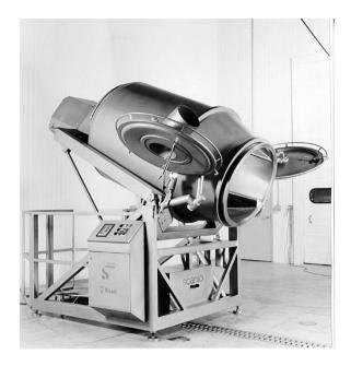
*Figure 15.4* Vacuum tumbler (in unloading position showing internal paddles) used for mixing marinade and other ingredients with larger meat particles or whole muscles. (Courtesy of Wolfking, Inc.)
