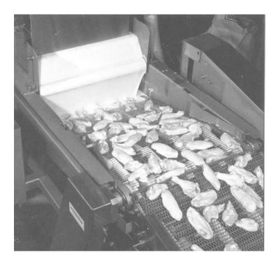
*Figure 13.13* Batter application on chicken wings using overflow system. (Courtesy of STEIN • DSI, a business of FMC FoodTech, Sandusky, OH.)
