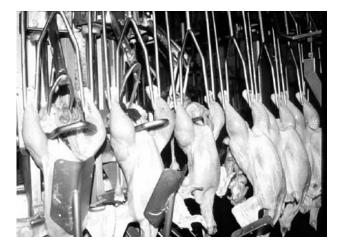
*Figure 3.11* Evisceration or drawing machine showing scoop withdrawing viscera from carcass. Visceral "package" can be seen hanging behind the fourth carcass from the left.
