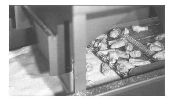
*Figure 13.15* Breader application on battered chicken wings. (Courtesy of STEIN • DSI, a business of FMC FoodTech, Sandusky, OH.)
