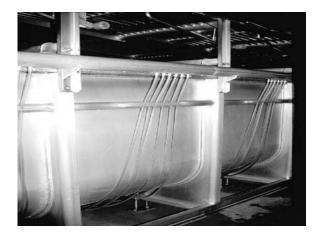
*Figure 3.18* Water-immersion chilling tank showing air hoses used to agitate the water with bubbles.
