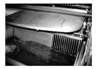
*Figure 3.16* Paddles in a chiller to move carcasses. Open side of paddle alternates between paddles to agitate the water.
