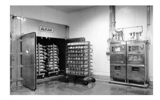
*Figure 15.15* ALKAR batch oven with DDC computer controls for cooking and smoking of poultry products. (Courtesy of ALKAR, A Division of DEC International, Inc., Lodi, WI).
