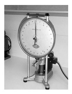
Figure 7.4 Warner-Bratzler shearing device.
