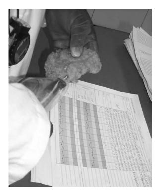
*Figure 18.4* A quality department technician checks cooked product temperature and records data on an X bar and R bar "rainbow" control chart.
