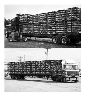
*Figure 2.7* Typical auto-dump coops (modules) being unloaded from the truck.
